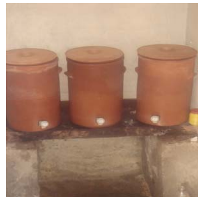
Colloidal silver filters placed in the primary school to treat water functioned well throughout the NHIP survey.
